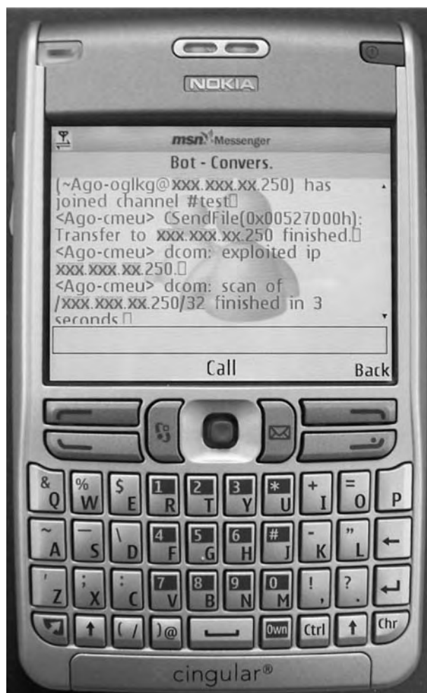
FIGURE 8.8 Using a Nokia smartphone to control an Agobot-based botnet. (Photo courtesy of Ruishan Zhang.)
